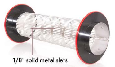
The solid steel slats on our wet tumblers are 1/8" in width compared to 1/4" on tumblers offered by our competitors. Having a thinner slat means less metal material and more open area, resulting in an overall increase in access to the blades by 50% when compared to the 1/4" wide standard dual-purpose tumbler.
