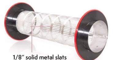
The solid steel slats on our wet tumblers are 1/8" in width compared to 1/4" on tumblers offered by our competitors. Having a thinner slat means less metal material and more open area, resulting in an overall increase in access to the blades by 50% when compared to the 1/4" wide standard dual-purpose tumbler.
